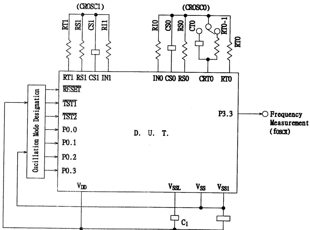
RTO, RTO-1 = 2k $\Omega$ /10k $\Omega$ /200k $\Omega$ RS0, RS 1 = 10k $\Omega$ RIO, RI 1 = 10k $\Omega$
