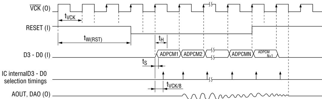
The  $\overline{VCK}$  clock rising and falling edges are reversed between the MSM5205 and the MSM6588, as indicated in DIFFERENCES BETWEEN MSM6585 AND MSM5205.
