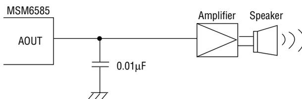
Even when the DAO pin is used, connect a  $0.01\mu\text{F}$  capacitor to the AOUT pin. This capacitor is used for the improvement of a voice quality.
