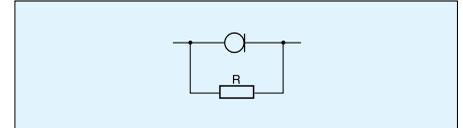
Compensative resistor is not necessary if the current value is less than 1 mA.
