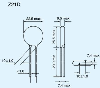
Crimped Leads and Taped
