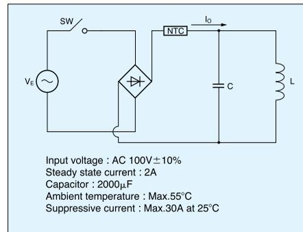
The most suitable power thermistor for the above circuit is required to fulfill the following terms and conditions.
