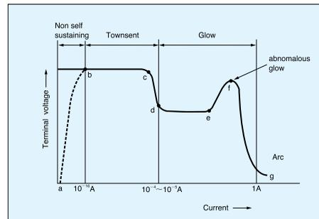
When the applied voltage across the GTA exceeds the breakdown voltage (sparkover voltage), the current through the GTA increases rapidly to value of several amps or greater. The rate of current rise and level to be reached are limited by the series impedance of the circuit. The voltage across the GTA at this time is very low with typical value of 20 to 30 volts.
