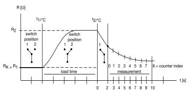
Change of resistance of a transformer winding in relation to the time factor.
