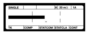
Example: bar indication with flashing-in of limits and comparator results
