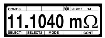
Example: main menu 1 with 5 1/2 reading of absolute value, additionally display of the measurement unit
