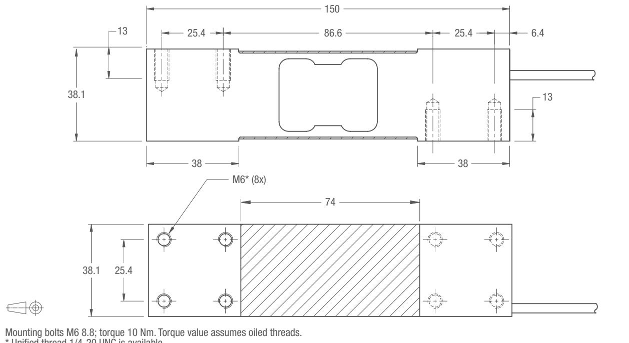
Mounting bolts M6 8.8; torque 10 Nm. Torque value assumes oiled threads.
