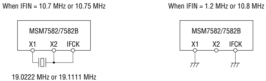
Figure 2 How to Use IFCK, X1, and X2
