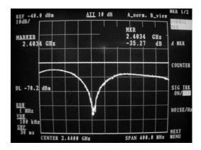
We can see that the antenna is correctly tuned at 2.4 GHz, and the reflected power is about 35 dB less than the case without the antenna. This is a good result.
