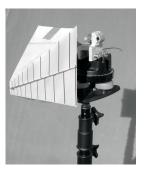
As third antenna we used an omnidirectional antenna. According to the datasheet it has a 4 dBi gain, but as explained the knowledge of the gain of this antenna is not necessary. A photo of the omnidirectional antenna mounted on the tripod is shown.
