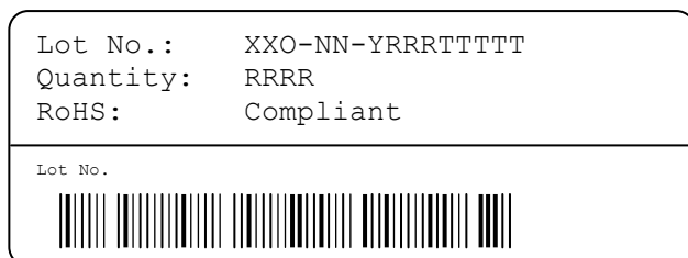
Figure 20: First label on reel: XX = Sensor Type (21 for SHT21), O = Output mode (D = Digital, P = PWM, S = SDM), NN = product revision no., Y = last digit of year, RRR = number of sensors on reel divided by 10 (200 for 2000 units), TTTTT = Traceability Code.
