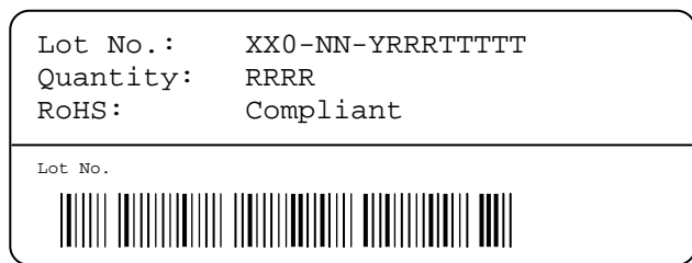
Figure 19: First label on reel: XX = Sensor Type (11 for SHT11), NN = Chip Version (04 for V4), Y = last digit of year, RRR = number of sensors on reel divided by 10 (200 for 2000 units), TTTTT = Traceability Code.
