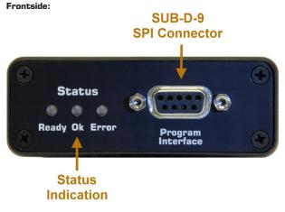
On the frontside there is a SUB-D-9 female connector for interfacing the PSO81 via SPI. 3 status LEDs are indicating the progress of the
