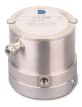
The LP 9000 Series accurately measure low differential or relative pressure of gases and liquids from 0.04 inH $_2$ O to 150 psid full scale. With a choice of current or voltage output, they are suitable for uni-directional, for example, 0 to 8 inH $_2$ O or bi-directional, for example, -8 to +8 inH $_2$ O.
