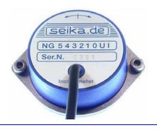
Inclinometers of high measurement accuracy with an integrated 4...20mA signal conditioner for inclination measurement in the ranges of ±10, ±30 and ±80 degrees
