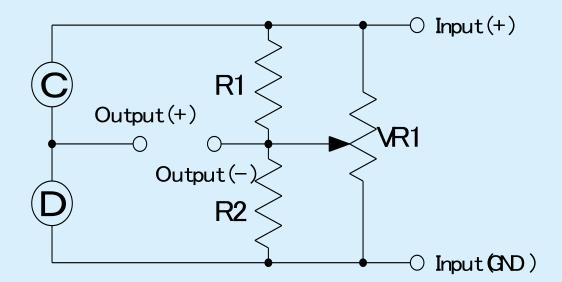
Pellistor Drive/Measurement Circuit: A simple Wheatstone Bridge to compare the resistance of two hot elements
