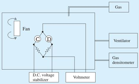
The test chamber should be constructed of glass, or another material known not to absorb gases.
