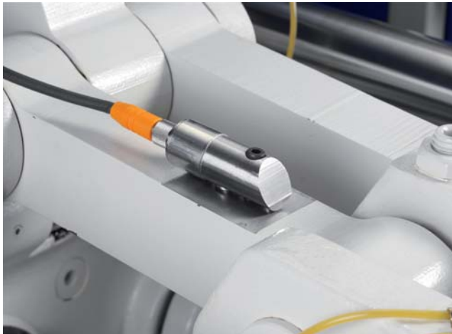
Fig. 8: Indirect force measurement on knuckle joint
