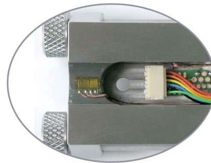
Fig. 3: Miniature connector inside load cell body
