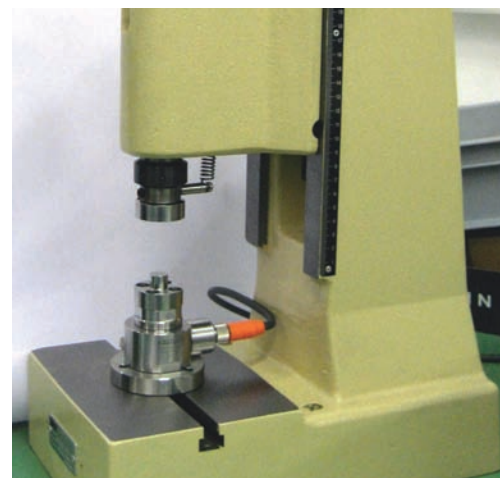
Fig. 4: Monitoring press-fitting forces on a knuckle-joint press
