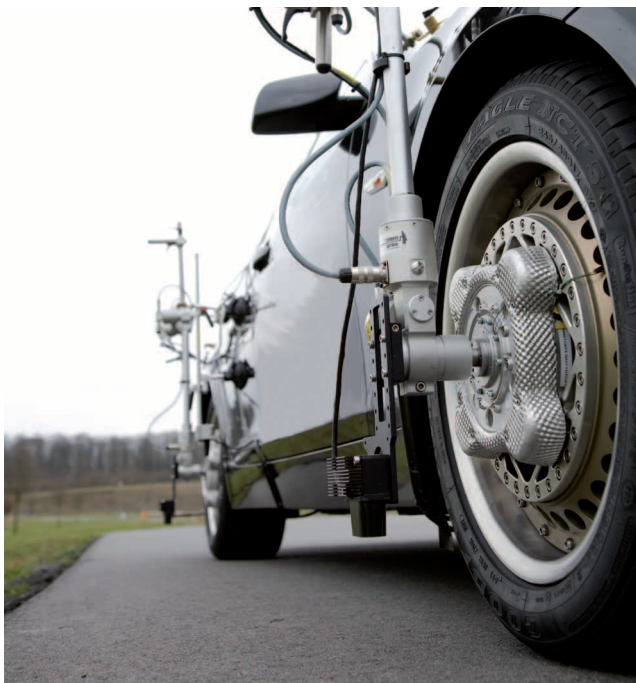
Fig. 2: RoaDyn® P650 with digital in-board transmission and RV-4 wheel vector sensor with Correvit®-SF sensor
