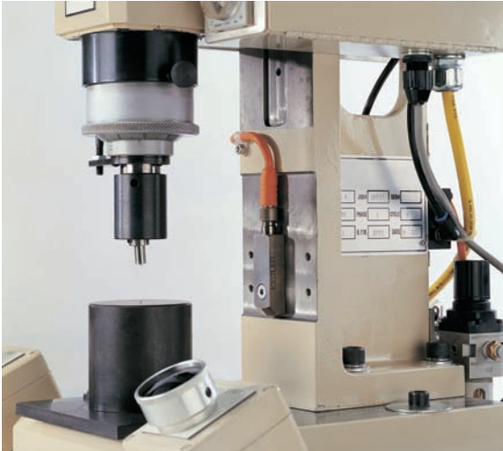
Fig. 1: Measuring force-proportional strain on a wobble riveting machine (C-form construction)
