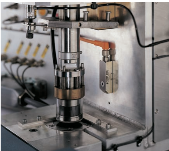
Fig. 2: Monitoring a metal forming press (C-form construction) against overload
