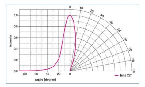
Figure 3 Opening Angle: Example RGB with Lens ⊳
