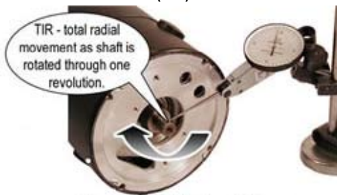
Figure 3 - Total Indicated Runout
