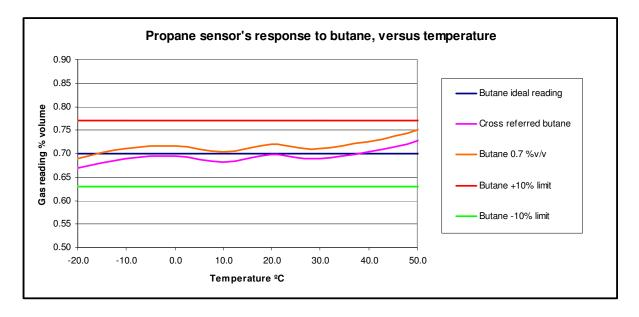
The above graph shows the output of a propane sensor, both with and without a cross-reference factor applied, against ambient temperature when tested with 0.7% volume butane.
