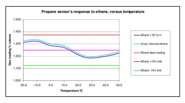
The above graph shows the output of a propane sensor, both with and without a cross-reference factor applied, against ambient temperature when tested with 1.25% volume ethane.
