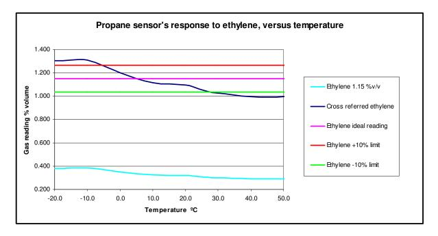
The above graph shows the output of a propane sensor, both with and without a cross-reference factor applied, against ambient temperature when tested with 1.15% volume ethylene.
