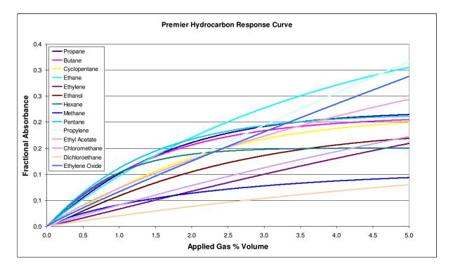
The above graph demonstrates the hydrocarbon sensor's fundamental response to a selection of gases, before any linearisation is applied.
