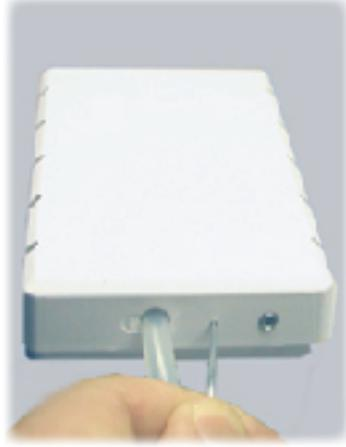
Use a long thin tool (such as a paper clip) to press calibration button.
