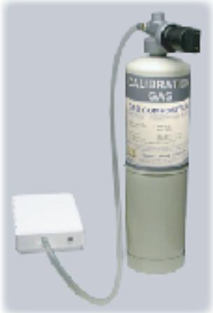
Remove Port Cover & Connect 2000 PPM CO<sub>2</sub> Calibration Gas
