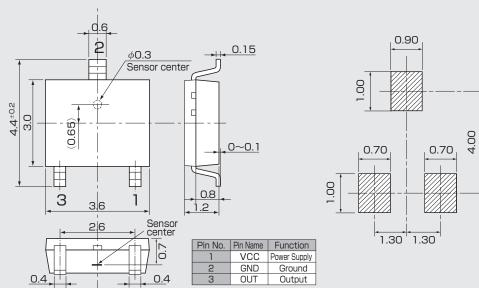
Note 1) The sensor center is located within the  $\phi$ 0.3mm circle.
