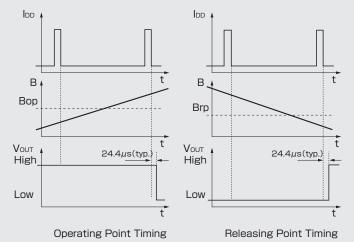
This Hall effect IC's output is held as internal data just before the internal circuit turns OFF (lob OFF). And after 24.4  $\mu$ s, the output changes.
