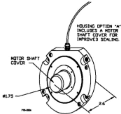
Housing style Option A completely encloses the motor shaft and eliminates access to the motor shaft. This housing style provides IP 65 protection.
