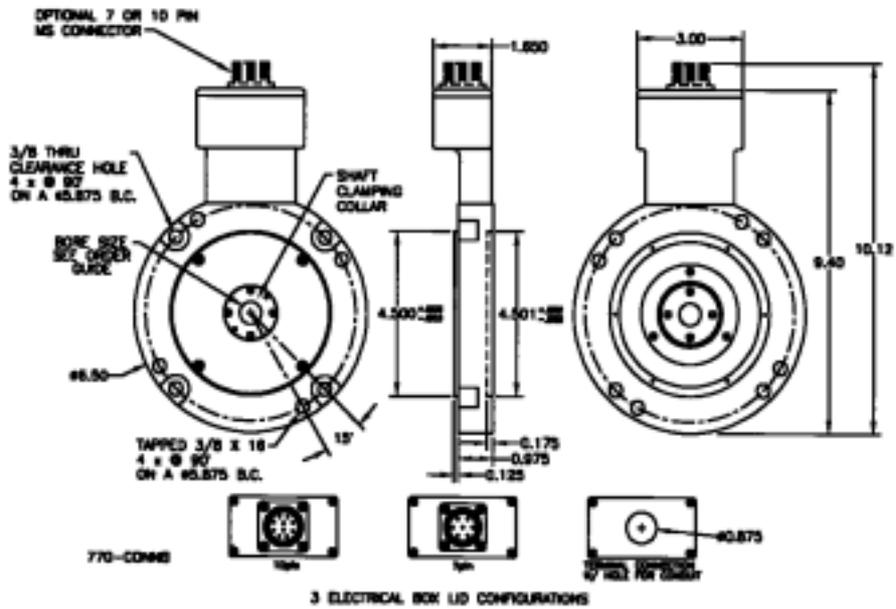
All dimensions are in inches with a tolerance of  $\pm 0.005$  or  $\pm 0.01$  unless otherwise specified
