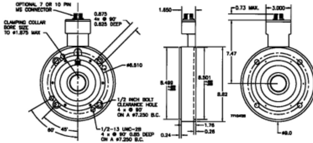
All dimensions are in inches with a tolerance of  $\pm 0.002$  or  $\pm 0.01$  unless otherwise specified
