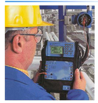
Direct connection of thermocouple compensation wires eliminates the need for special connectors. The cold junction temperature is continuously monitored and compensated for, even under the transient conditions experienced by a field calibrator. This is the most reliable and accurate cold junction compensation method found in a portable field calibrator.
