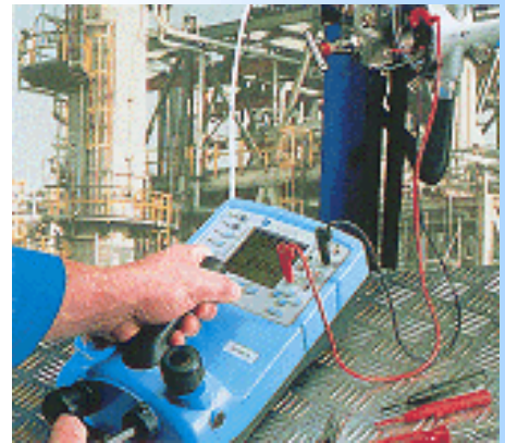
DPI610 Portable Pressure Calibrator in action.
