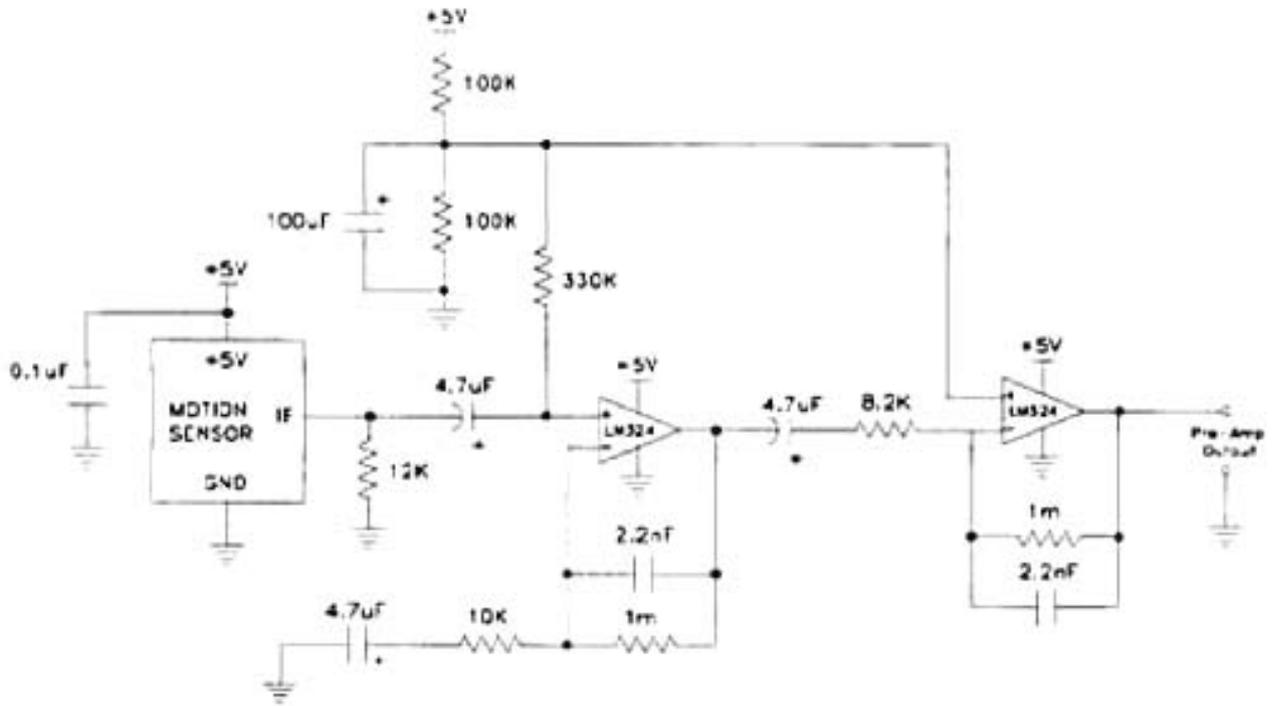
**Annex 3: Amplifier Circuit (Pulse operation, PRF =2 KHz, Duty Cycle = 4%)**
