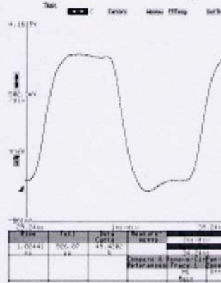
Fig. 6. T3492-125 M with 15 pf load. Rise time is 1.02 ns. Fall time is 0.96 ns. Duty cycle is 48.7%. Readings taken at 3.3V.
