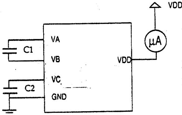
Note 9 : Measured by the test circuit while "0" is being displayed after auto - clear operation and while key is not being depressed.
