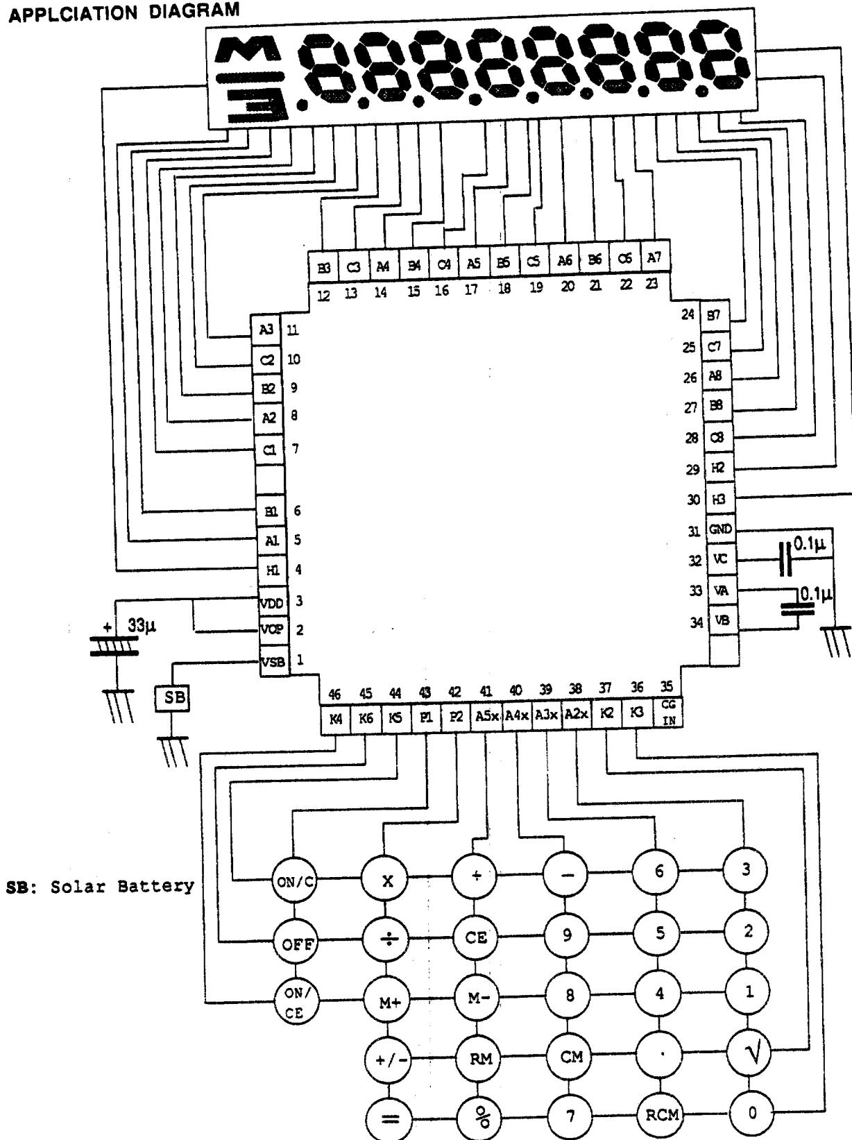
Note : Chip substrate must be floating or connected to GND.
