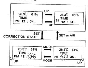
When the <UP> switch is pressed in normal state, the time system is exchanged (12-hour/24-hour).
