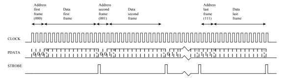
Figure 3. Serial data transfer (full configuration).
