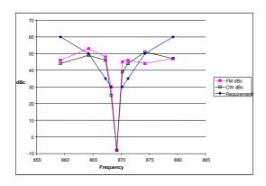
IF = 200 kHz, Separation = 40 kHz. Data rate = 1.2 kbit/s. Interfering signal is CW (no modulation) or FM modulation.
