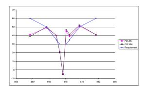
IF = 455 kHz external, Separation = 12 kHz. Data rate = 1.2 kbit/s. Interfering signal is CW (no modulation) or FM modulation.
