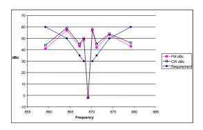
IF = 60 kHz, Separation = 20 kHz. Data rate = 1.2 kbit/s. Interfering signal is CW (no modulation) or FM modulation.
