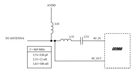
Figure 8. Input/output matching network.
