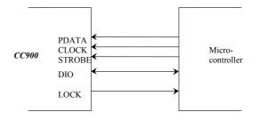
Figure 6. Microcontroller interface.
