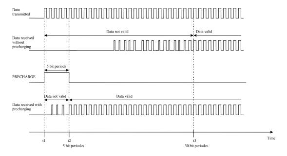
Figure 10: Demodulation using precharging.
