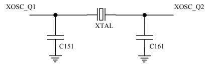
Figure 10. Crystal oscillator circuit.
