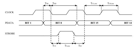
Figure 4. Timing diagram, serial interface.
