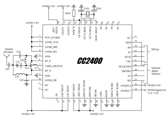
Figure 3 Typical application circuit with discrete balun for interfacing single-ended antenna
