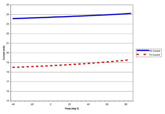
Figure 24 Typical RX and TX current vs. temperature
