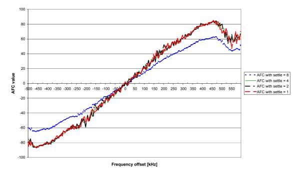
Figure 21. AFC value vs. frequency offset
