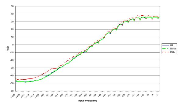
Figure 22. Typical RSSI value vs. input power
