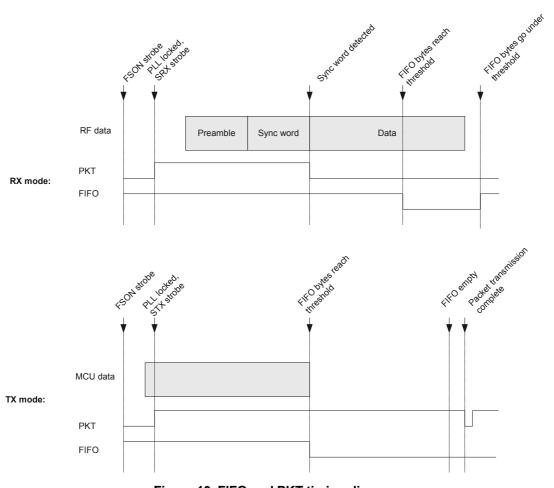
Figure 10. FIFO and PKT timing diagram
