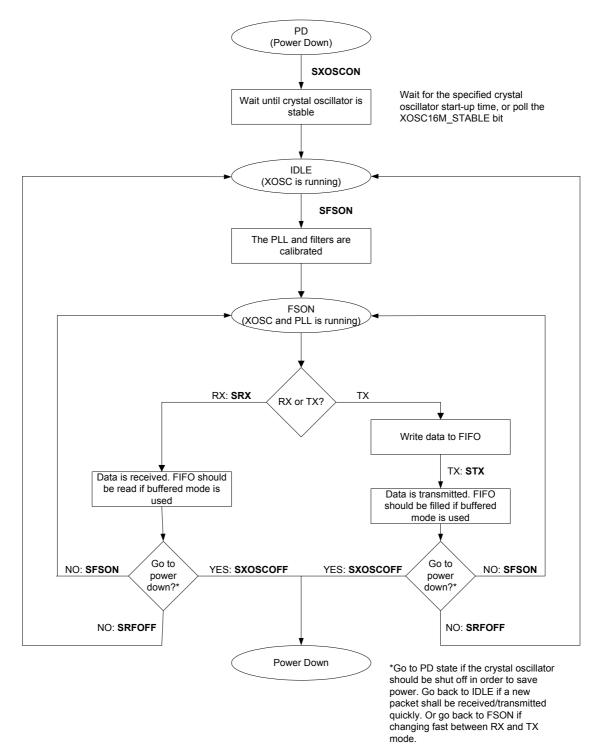
Figure 17. Sequence for activating RX or TX mode
