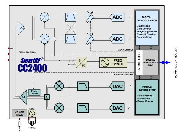
Figure 2. CC2400 simplified block diagram
