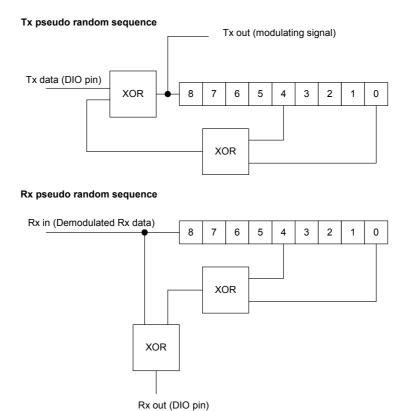
Figure 34. PN9 pseudo random sequence generator in TX and RX mode
