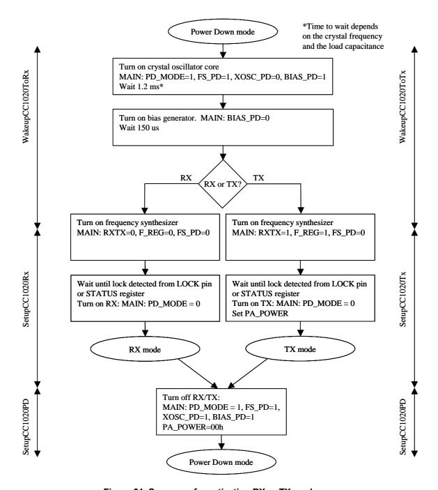
Figure 31. Sequence for activating RX or TX mode
