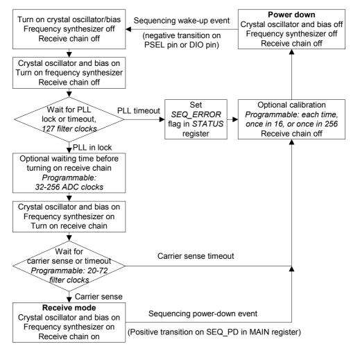
Figure 21. Automatic power-up sequencing flow chart
