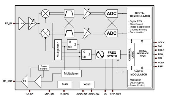
Figure 2. CC1021 simplified block diagram
