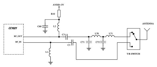
Figure 25. Input/output matching network
