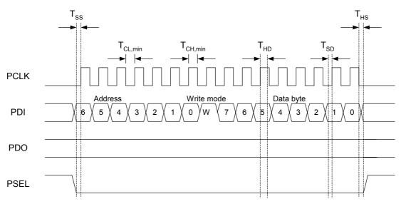
Figure 7. Configuration registers write operation
