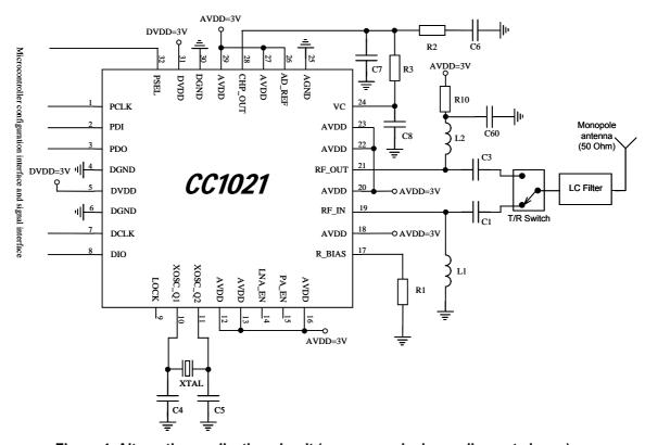
Figure 4. Alternative application circuit (power supply decoupling not shown)
