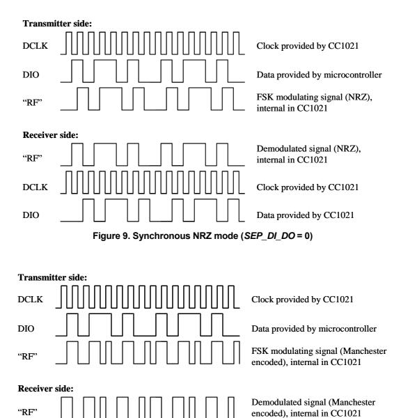
Figure 10. Synchronous Manchester encoded mode (SEP\_DI\_DO = 0)
