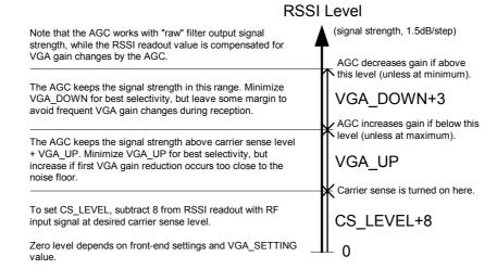
Figure 20. Relationship between RSSI, carrier sense level, and AGC settings CS\_LEVEL, VGA\_UP and VGA\_DOWN
