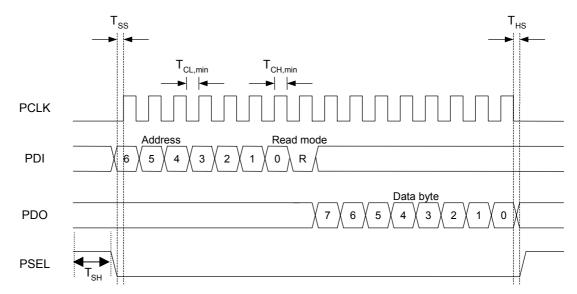
Figure 8. Configuration registers read operation
