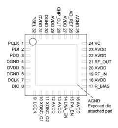
Figure 1. CC1021 package (top view)
