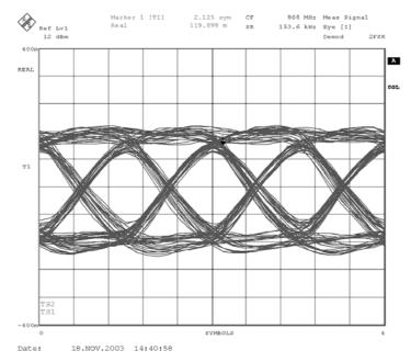
Figure 22. GFSK eye diagram. 153.6 kBaud, NRZ, ±79.2 kHz frequency deviation.
