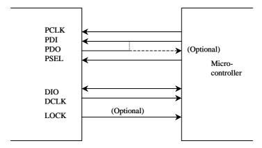
Figure 6. Microcontroller interface
