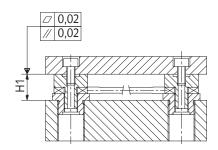
Mounting of SLS quartz force links in force plates or dynamometers with extremely low construction height.
