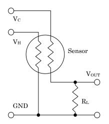
Pins I and 3 on the TO-39 header are attached to the heater. Apply  $V_{H}$  across these pins.
