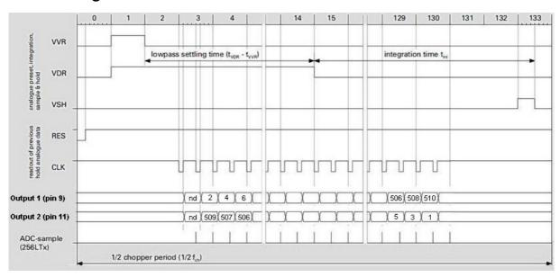
The 510 channel line sensor contains two multiplexed analogue outputs, each one providing data from 255 channels. The first output (pin 9) provides data from all the even numbered pixels, counting upwards from 2 to 510. The second output (pin 11) provides data from all the odd numbered pixels, starting at pixel 509 and counting downwards to pixel 1. The clock diagram above shows which pixel numbers are available from each output as the device is clocked.
