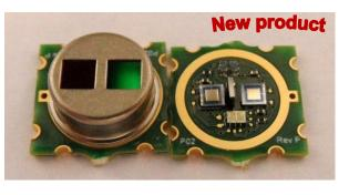
uniquely high standards of performance and also delivers higher levels of EMC protection. An additional feature is that the sensor elements have integrated temperature sensors on each channel to provide the most accurate possible temperature reference and further simplify product development.
