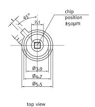
UVC-only SiC based UV photodiode A = 1,0 mm<sup>2</sup>
