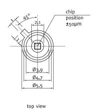
UVB-only SiC based UV photodiode A = 1,0 mm<sup>2</sup>
