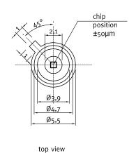
UVA-only SiC based UV photodiode A = 0,50 mm<sup>2</sup>
