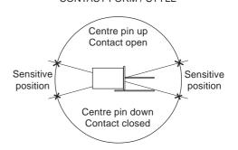
Contact Form/Style: Switch types CW1300 may have a normally open or closed contact depending on the positioning of the switch. These switches have a change in sensitivity depending on the switch position.
