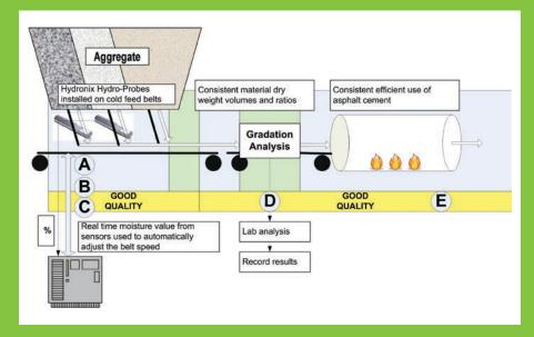
moisture. Taking the case of PennDOT officials reporting up to 7 percent moisture in the RAP piles during the rainy season, this would equate to 14 tons of water having to be evaporated per hour from a plant producing 200 tons per hour. Without accurate moisture compensation this would also equate to 14 tons of lost yield in comparison to asphalt cement (AC) use and also a reduction in plant output of 14 tons per hour.
