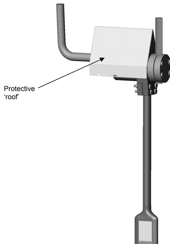
Figure 5 - Protective 'roof' placed over the sensor body
