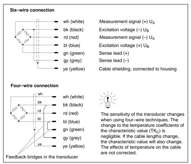
Fig. 6.1 C2 pin assignment; cable lengths 6m
