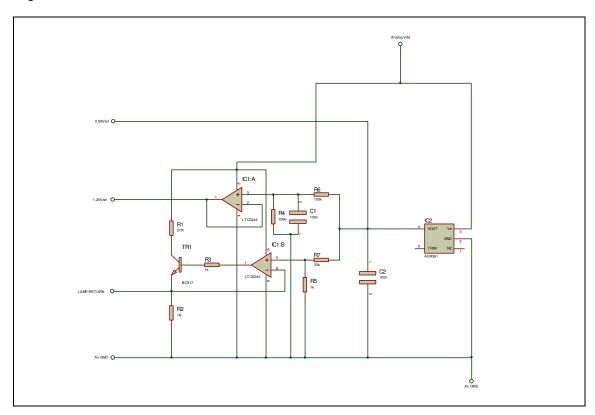
Fig.2: Suggested IR source constant current circuit and reference generator.
