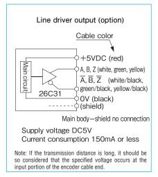
A capacitor  $(0.1 \mu F)$  is connected between OV and FG (frame ground).
