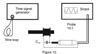
At the point where the voltage of the RF signal at the probe drops by 3 dB, the two frequencies can then be measured. The difference between these two frequencies is called the bandwidth  $BW_A$  of the antenna circuit. As the value of the capacitor  $C_{res}$  in the antenna circuit is known, it is easy to compute the resonant resistance according to the following formula:
