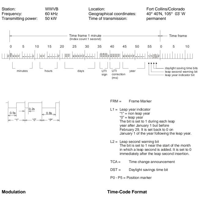
The carrier amplitude is reduced by 10 dB at the beginning of each second and is restored within 500 ms (binary one) or within 200 ms (binary zero) or within 800 ms (position-identifier marker or frame reference marker).
