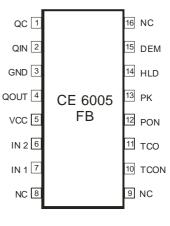
Figure 3. Pin layout SSO16
