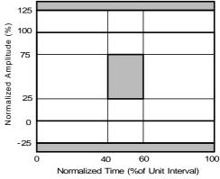
Figure 1. Transmitter Eye Diagram
