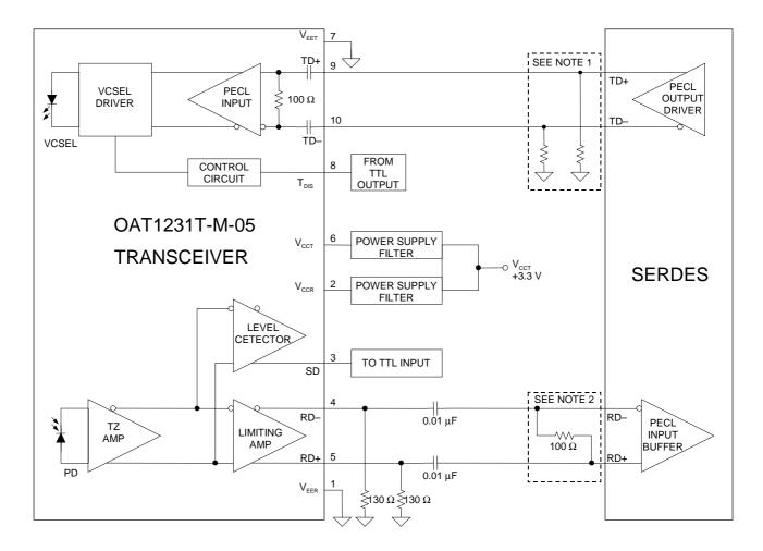
Figure 3. Example of TD+/- and RD+/- Termination
