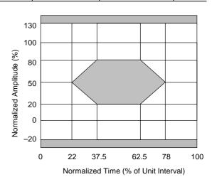
Figure 1. Transmitter Eye Diagram
